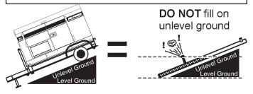
Figure 22. Only Fill on Level Ground
